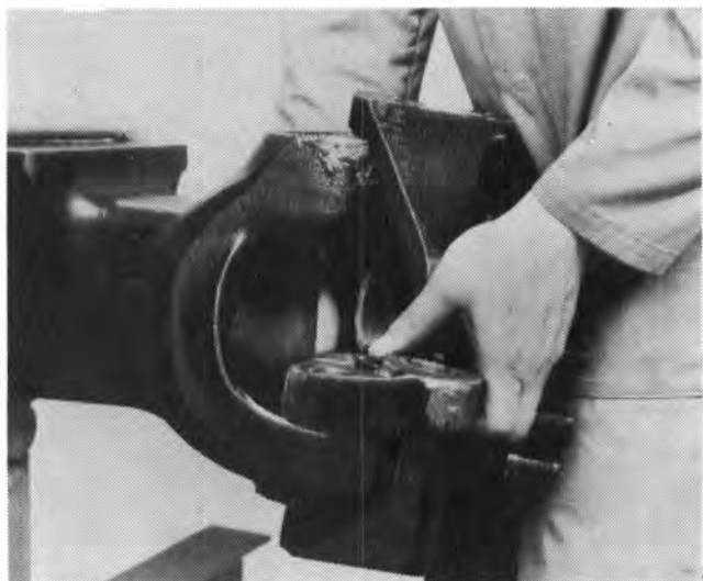
4. Tip the steering knuckle slightly and remove from housing yoke.
