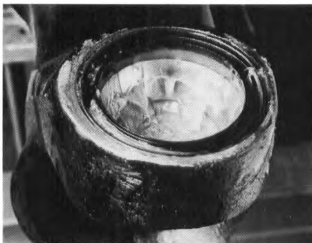
7. Inspect bearing cup and seal; replace if necessary.
