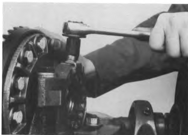
1. Remove adjusting nut lock from bearing caps.
