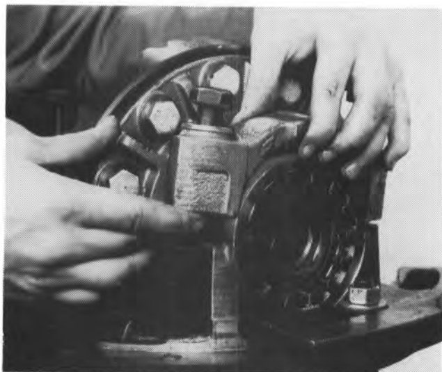
3. Remove bearing cap retaining bolts.
