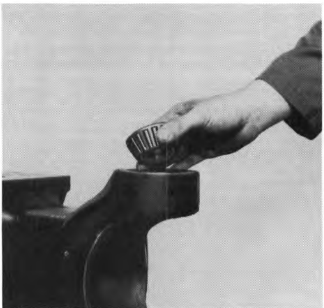
5. Inspect bearing cone and replace if necessary.
