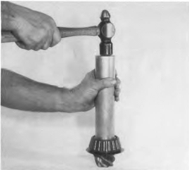
4. Assemble inner bearing cone (and a slinger if used) on pinion; place bearing installer over pinion shaft as shown. Drive bearing on shaft until it is completely seated.
