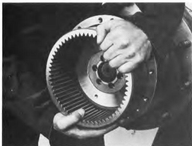
C. Remove planetary ring gear, brake piston and wheel retainer as one unit.
