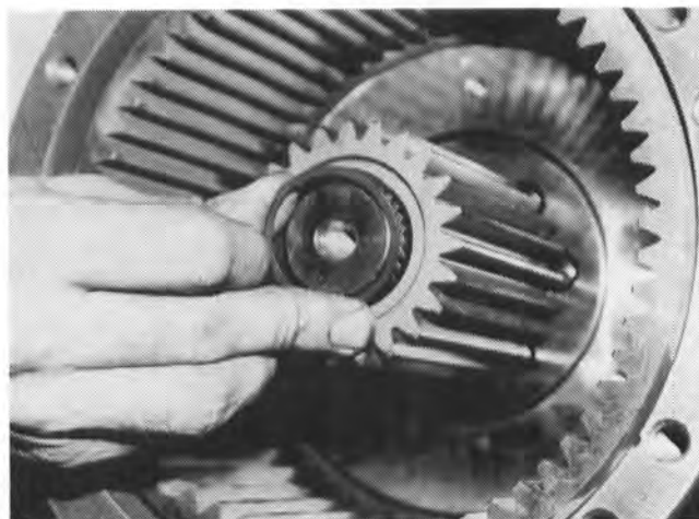
12. Install snap ring into groove on outboard end of outer shaft.
