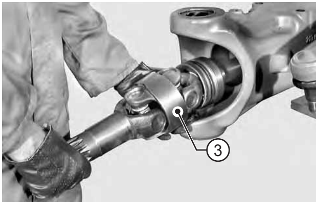
FIGURE 2: Extract the whole twin u-joint (3).
