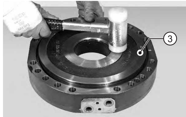
FIGURE 25: Using a plastic hammer, install the piston (3) into the cylinder (17).
