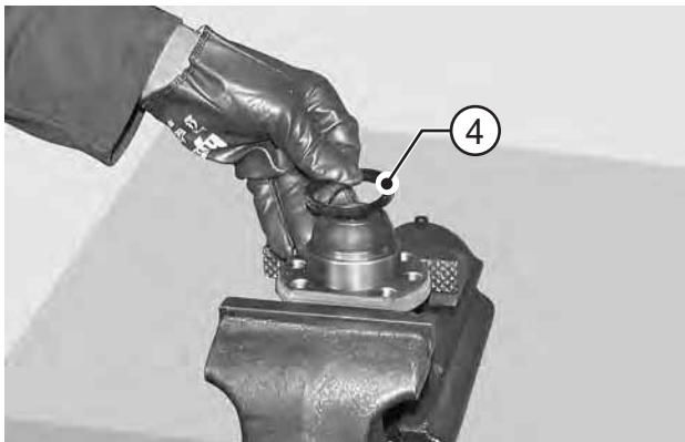
FIGURE 8: Remove the dust ring from the lower pivot pin (4).
