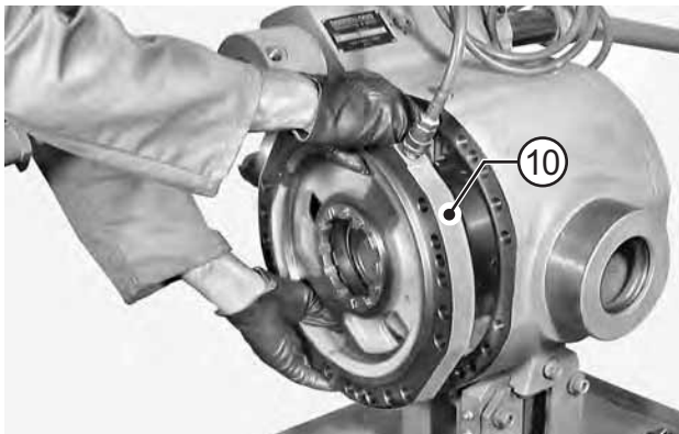
FIGURE 8: Introduce low-pressure compressed air through connection "B" and make sure that the lock control piston comes out at end of stroke. Remove safety studs, rotate cover (10) to an angle of about 45°, and remove cover.
