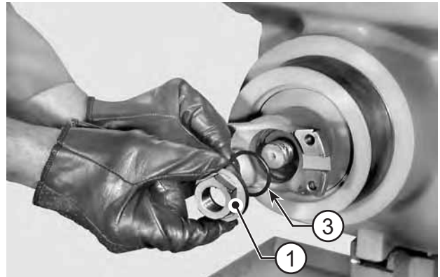
FIGURE 4: Remove nut (1) and o-ring (3).
