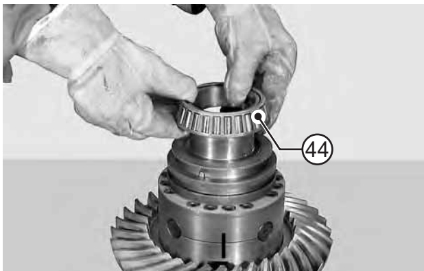
FIGURE 28: Heat bearing (44) to approximately 194 °F [90 °C] and install on the differential.
