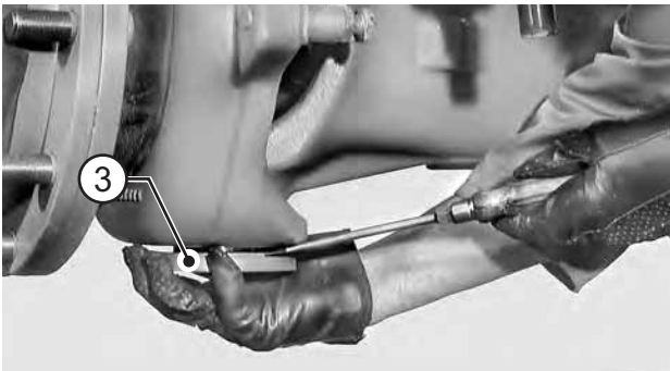
FIGURE 3: Insert a screwdriver or lever alternately in the slots provided and pry out the lower pivot pin (3) along with the dust ring (4).
