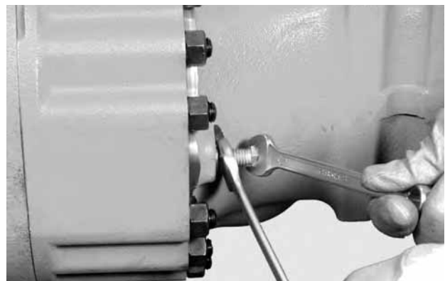
FIGURE 6: Lock into position with nuts (22).
