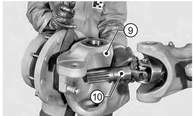
FIGURE 6: Remove the complete steering case (9) by drawing it out from the twin joint (10).
