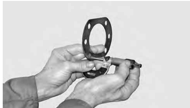
FIGURE 20: Calculate the average of measurements taken and subtract 0 - 0.1 mm from the resulting measurement until you have rounded off to the lower decimal figure. Make up the pack of shims choosing among available shims.
