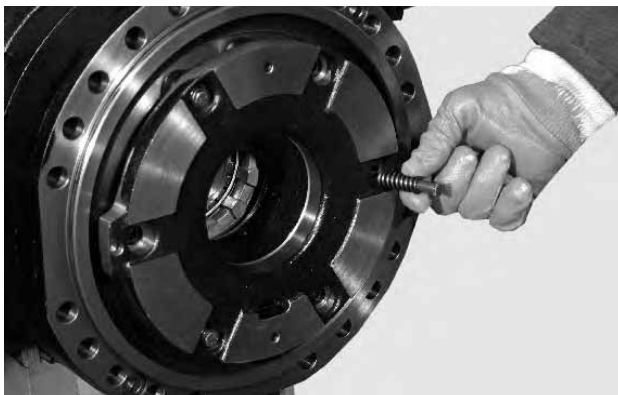
FIGURE 15: Remove the reversal springs (9) and screws (10).
