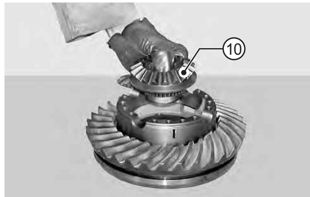
FIGURE 10: Install planetary gear (10).
