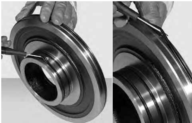
FIGURE 23: Fit o-ring (2) and (4) and anti-extrusion ring (18) onto the piston (3).
