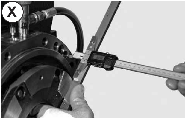
FIGURE 40: Take the measurement from the surface of the intermediate disk to the cover sealing surface with 20 - 35 bar of pressure introduced. EXAMPLE: 30,6 mm
