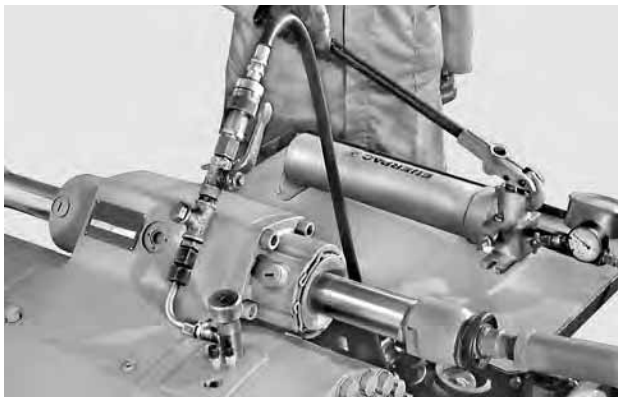
FIGURE 37: ADJUSTING BRAKES When adjusting the brakes, connect a hydraulic pump to the access hole of the negative brake and introduce pressure at 20 - 25 bar to release the brake disc.
