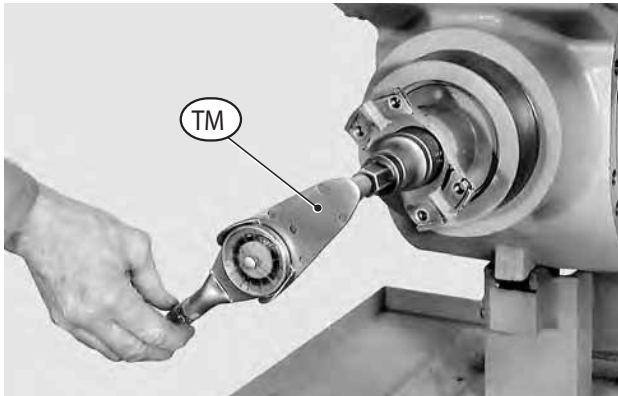
FIGURE 34: Apply torque meter TM to pinion nut and check that torque will increase by 20 - 40 Ncm as a result of differential bearing preload.
