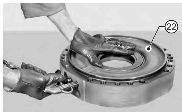
FIGURE 18: DISASSEMBLING THE BRAKE PISTON Gently introduce low-pressure compressed air through the connection of the working brake line and eject the complete piston (22).
