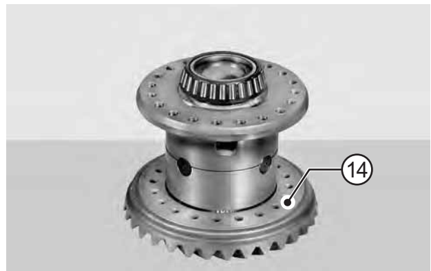
FIGURE 12: Remove the ring gear (14).
