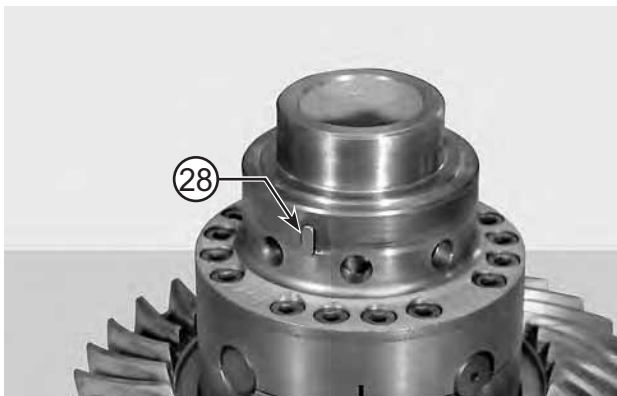
FIGURE 21: Only if necessary, remove guide key (28) from coupling (25).
