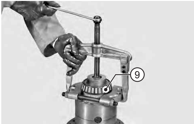
FIGURE 14: Using a separator and a puller, remove bearing from non-ring gear side.
