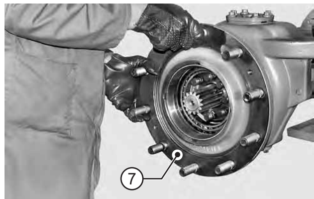
FIGURE 31: Install the wheel hub (7) onto the steering case (3).
