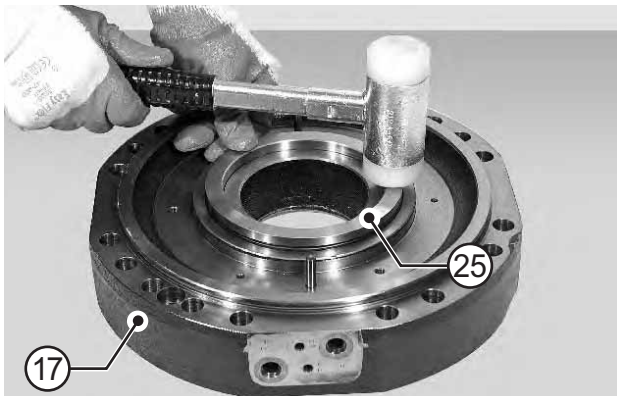
FIGURE 29: Using a plastic hammer, install the piston (25) into the cylinder (17).
