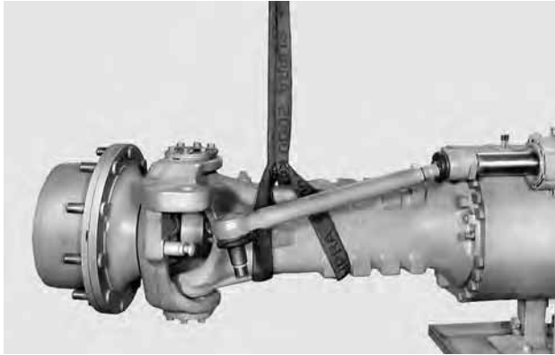
FIGURE 1: Remove the arms, negative brake cylinders and differential unit. For details, see CHECKING WEAR AND REPLACING THE BRAKING DISCS p. 17 and DIFFERENTIAL UNIT p. 73.
