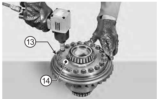
FIGURE 11: Loosen and remove the check screws (13) of ring gear (14).
