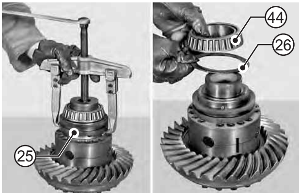
FIGURE 19: DISASSEMBLING THE DIFFERENTIAL GEAR With a puller applied under coupling (25), remove bearing (44) and shoulder (26) for coupling (25).
