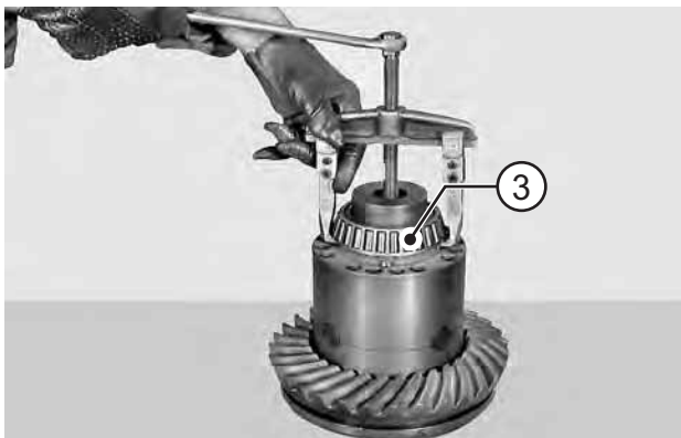
FIGURE 2: Using a puller, remove bearing (3).
