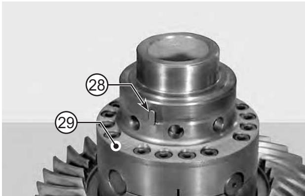
FIGURE 26: IF DIFFERENTIAL HAS BEEN DISASSEMBLED Assemble the differential unit (29). For details, see DIFFERENTIAL UNIT p. 73 in the first part of the manual. Put the guide key (28) of coupling (25) in place.
