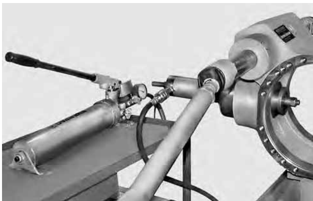
FIGURE 19: Connect the tension bar to the press and push the thrust blocks of bearings (9) and (10) into their seats. Disconnect from the press and remove tension bar and drivers.
