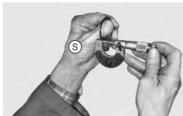
FIGURE 17: Subtract 0.05 - 0.07 mm from the resulting S value, until the value is rounded off to the lower 5/100. EXAMPLE: S = 0.82 = 0.75 mm. Make up the pack of shims "S".
