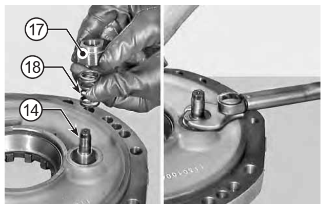
FIGURE 31: Fit spring (18) and ring nut (17) on piston (14). Tighten the ring nut by a few turns. Apply a coat of Loctite 242 to the ring nut and tighten to a maximum torque of 50 N·m.
