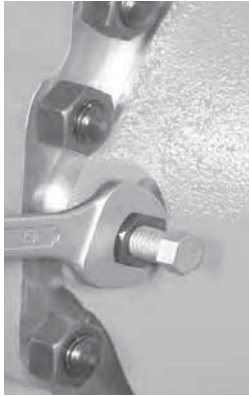
FIGURE 1: Loosen nuts (22) of screws (23) provided for the mechanical and manual release of the braking units, then move the nuts backwards by approximately 8 mm.
